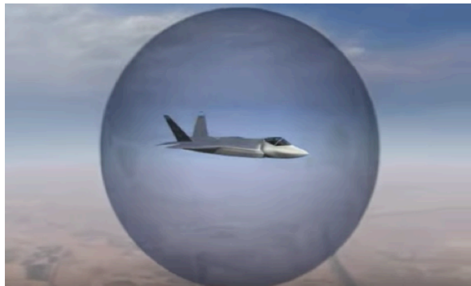
The DAS System enables complete spherical sensor coverage around the F-35, able to detect a wide-array of threats ranging from tactical ballistic missile launch to SAM system, as well as enemy aircraft 70
